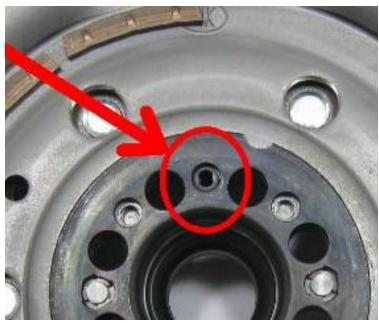
On the rear of the flywheel the dowel is only located where indicated.
