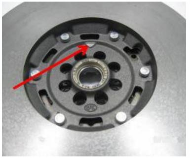
The triangular shaped mark on the flywheel face must be in line with the dowel on the crankshaft.
