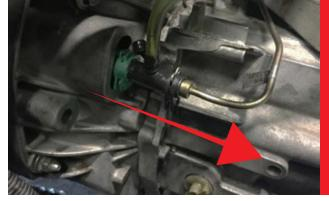
Fill the reservoir with fluid and allow the fluid to gravity bleed. Using a hand slowly depress the pedal by  $\frac{3}{4}$  stroke and back 3-4 times.
