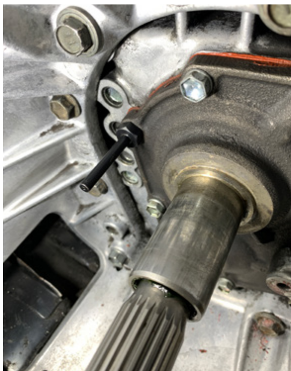
CSC guide pin/locking tab install example
