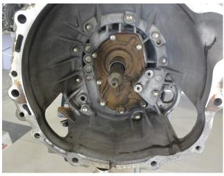
3. Mount the new pivot ball bracket onto the transmission using the supplied M8 bolts with spring washers and thread lock. Ensure that the bracket is mounted in the correct orientation with the cut-out sections facing towards the input shaft. Torque the bolts to 32Nm.
