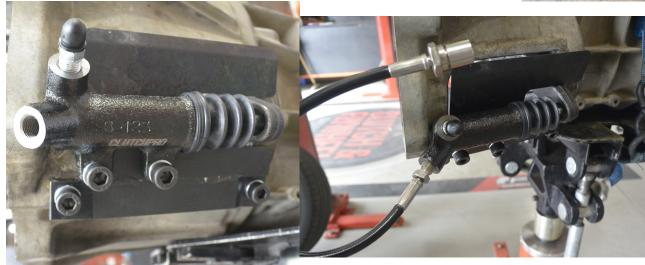
11. With the clutch installed, the transmission can be carefully mounted to the engine. Connect the braided line to the existing hard line.
