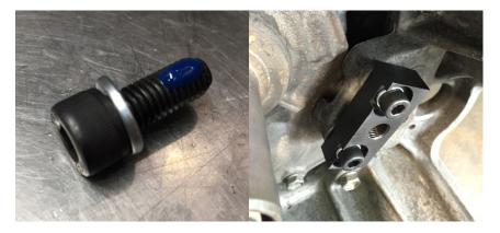
4. Mount the new pivot ball onto the pivot ball bracket using thread lock. Torque it to 70Nm.
