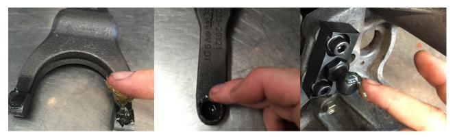
7. Mount the release bearing carrier onto the fork by tilting the fork underenath the clip, so the clip sits in the grooves of the fork.
