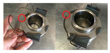
6. Lubricate all of the fork contact points using high temperature bearing grease. This includes where the fork contacts the bearing carrier, pivot ball and push rod.
