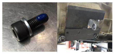
10. Mount the slave cylinder onto the adaptor plate using the M8 bolts, spring washers and thread lock. Torque the bolts to 32Nm. Fit the new braided clutch line to the slave.
