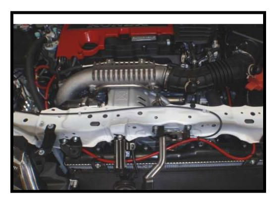
10. Undo the hose clip and pull away from the pipe, undo the four bolts holding the pipe work in position and one bolt at the back holding the inlet pipe in position. Remove the small rubber hose to the left.
