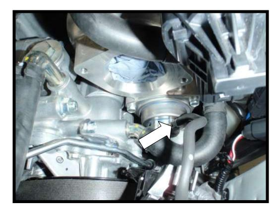
13. Install the blanking plate and refit the inlet pipe in reverse order of removal.
