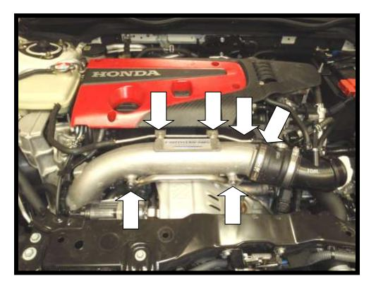
11. Undo the two bolts holding the plastic clip in position and move it as far out of the way as possible. Undo the two bolts from the flange of the pipe and remove the part from the vehicle.
