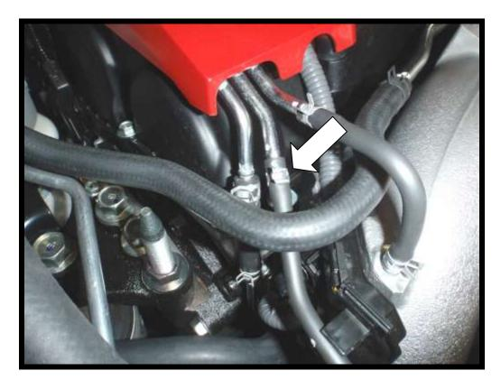
9. Feed the silicone hose through the slam panel, across the radiator and back to the new dump valve. (Additional parts removed to illustrate). Secure each connection with the cable ties provided.
