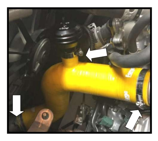
8. Disconnect the OEM Dump valve signal hose and connect the length of silicone hose provided to the vacuum source.
