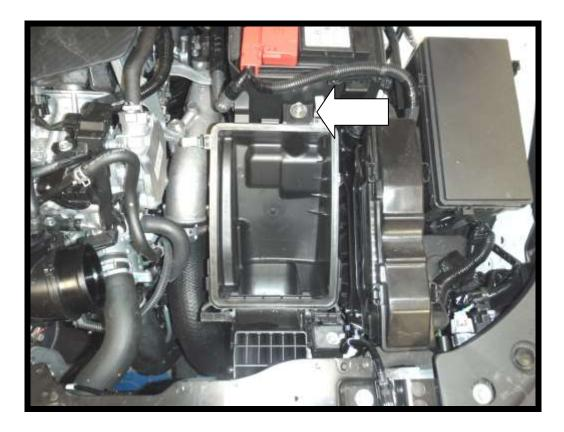
6. Using a 7mm hose clamp drive undo 2x hose clamps.
