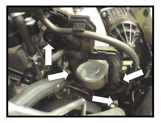
12. Unclip the vacuum hose, undo the three bolts and remove the OEM dump valve.
