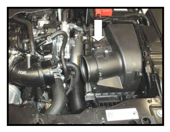
5. Using a 10mm socket and suitable ratchet undo the 1x bolt. Pull the airbox up firmly to remove it from the vehicle.
