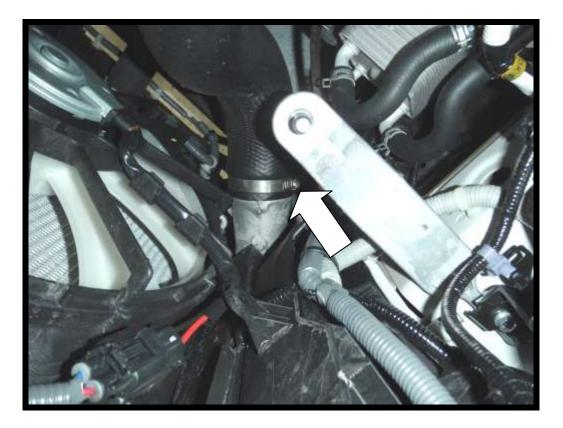
7. Fit the silicone hose provided and secure with 2x suitable hose clamps. Install the Forge Dump valve into the 25mm port and secure with a suitable hose clamp.
