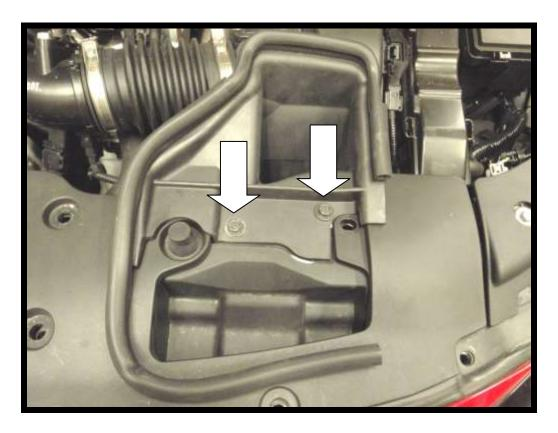
2. Unclip the intake scoop from the airbox inlet spout.
