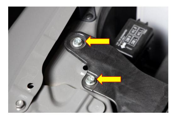
**3.** Locate the two M6 fasteners attaching the air box to the engine, remove these with a 10mm spanner. There is a wiring loom which is attached to the air box use a trim tool or flat blade screwdriver to release this loom.
