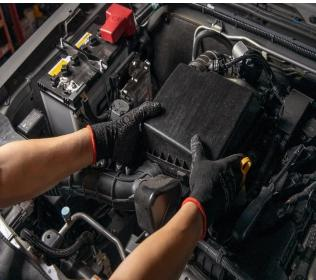
**5.** The hose clamp holding the turbo intake pipe also needs to be slackened off with an 8mm socket or flat blade screwdriver. Remove the sensor and oil breather hose from the turbo intake pipe, these will just pull out. Remove the rubber hose from the throttle body.
