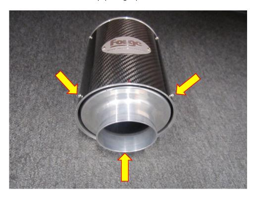
**8.** With the filter removed from the canister, fit the L bracket, two M6 washers, two M6 nuts and the rubber anti-vibration bush from the kit. Insert the larger thread of the anti-vibration bush into the 6mm hole in the carbon canister, use one of the washers and nuts to secure it into place. You will need a 10mm spanner to tighten them.
