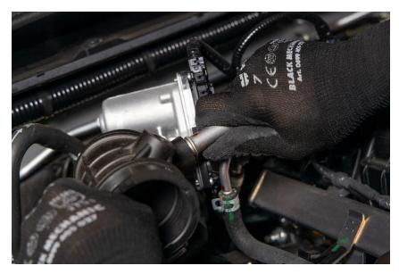
**6.** Fit the smaller silicon hose from the FMINDK34 kit to the throttle body. Use the 40-60 hose clamp for the throttle body side and the 70-90 for the air filter side of the hose. The sensor and oil breather which was removed in the previous step can now be re installed in the same positions as the OE hose, these just push into place. Use a 7mm socket and rachet or flat blade screwdriver to tighten both hose clamps.
