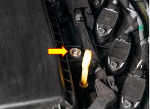
**4.** Undo the hose clamp securing the rubber hose to the air box. Use an 8mm socket and rachet or a flat blade screwdriver to do this. The air box can now be removed from the engine bay.
