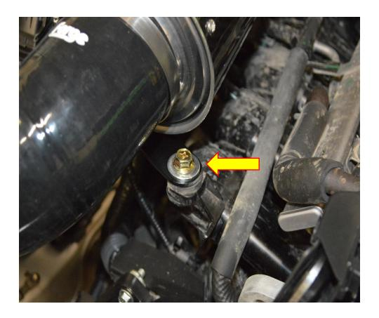
10. Place the Forge air scoop from the kit into place by lining up the two 6mm holes in the air scoop with the two threaded holes in the slam panel of the vehicle. Use the two M6x10 fasteners and the two M6 washers to fix it into place. Use a 10mm spanner to do this.
