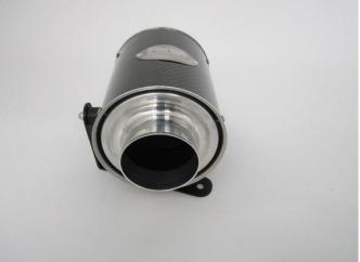
**9.** Fit the carbon filter to the silicon hose installed earlier, Use the M8 fastener, two M8 washers and M8 nut to fasten the bracket attached to the filter to the old mounting point of the OE filter box. Use a 13mm socket and spanner to tighten them up, you will now be able to tighten the hose clamp for the silicon hose with a 8mm socket or flat blade screwdriver.
