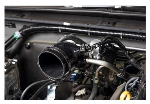
**7.** Before fitting the air filter, you must first attach the mounting bracket. Use a Philips screwdriver to release the three fasteners which hold the alloy spinning in place.
