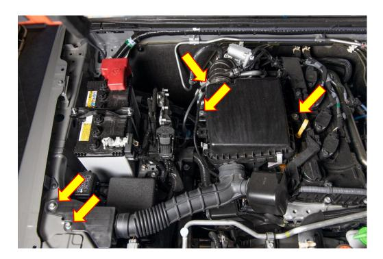
**2.** Remove the two M6 fasteners attaching the air scoop to the slam panel, use a 10mm socket and drive to do this.
