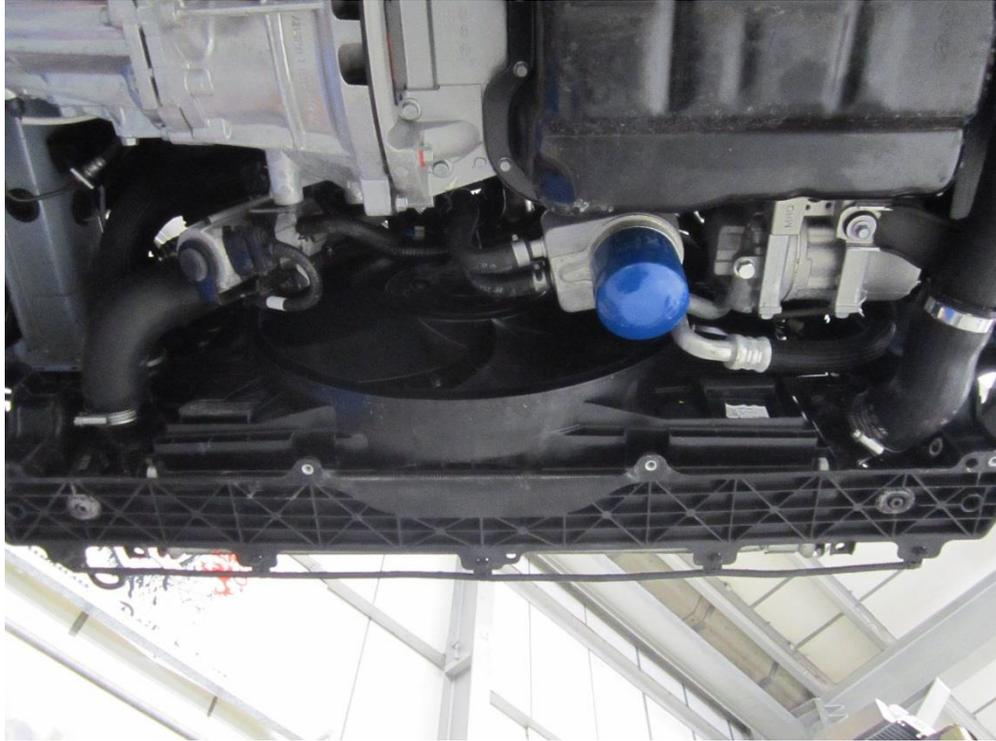
12. Finally, to remove the intercooler undo the 4 fasteners attaching it to the car, remove them using a 10mm socket and ratchet drive. The intercooler can now be removed from the vehicle.
