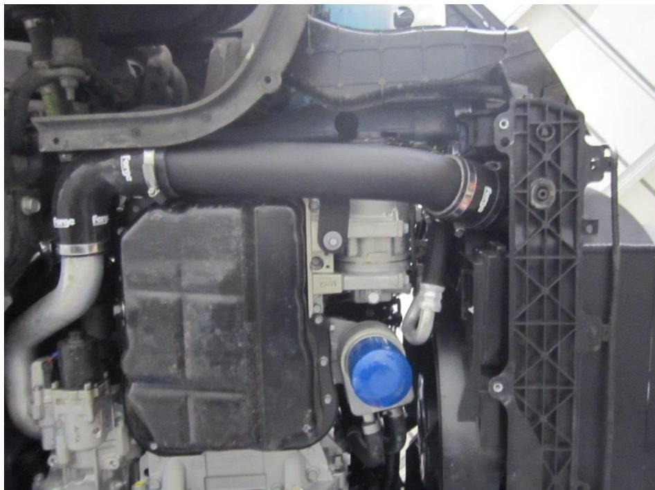
19. Now fit the near-side hose to the intercooler. This is also secured with 7mm hose clamps, the same as the off-side hoses.
