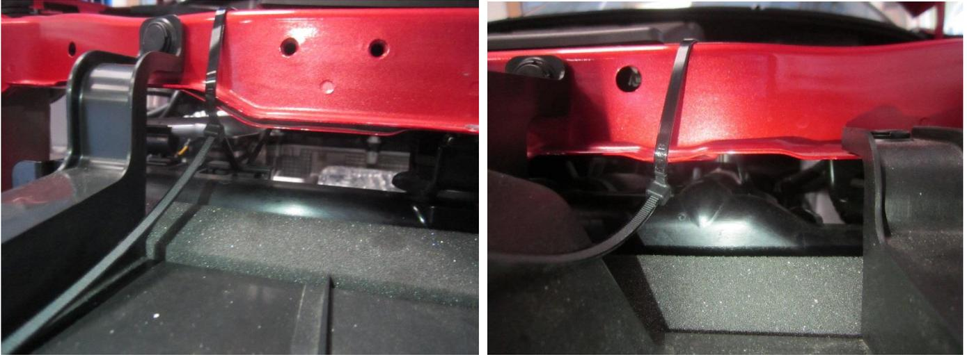
10. There is a black metal mounting bracket which needs to be removed, there are four 10mm fasteners that hold it in place use a 10mm socket and ratchet to remove them and the bracket will free from the vehicle.
