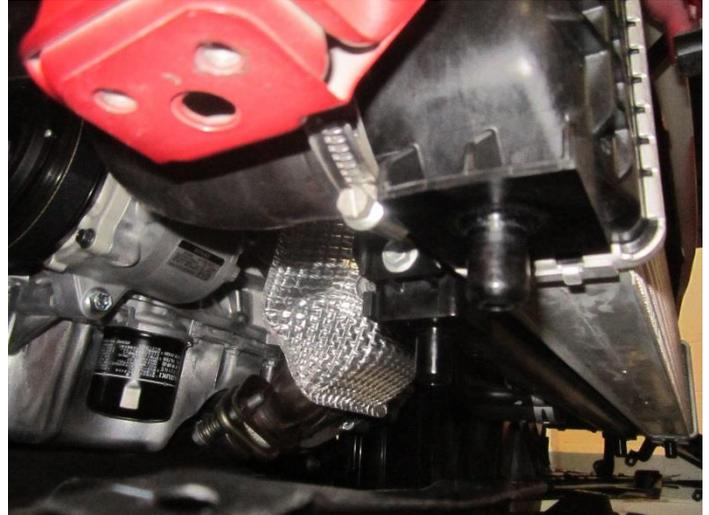
12. The final stage for removal of the OE inter cooler is to remove the two 10mm fasteners attaching the intercooler to the vehicle, use a 10mm ratchet and drive to release fasteners and you be able to release the inter cooler from the vehicle.
