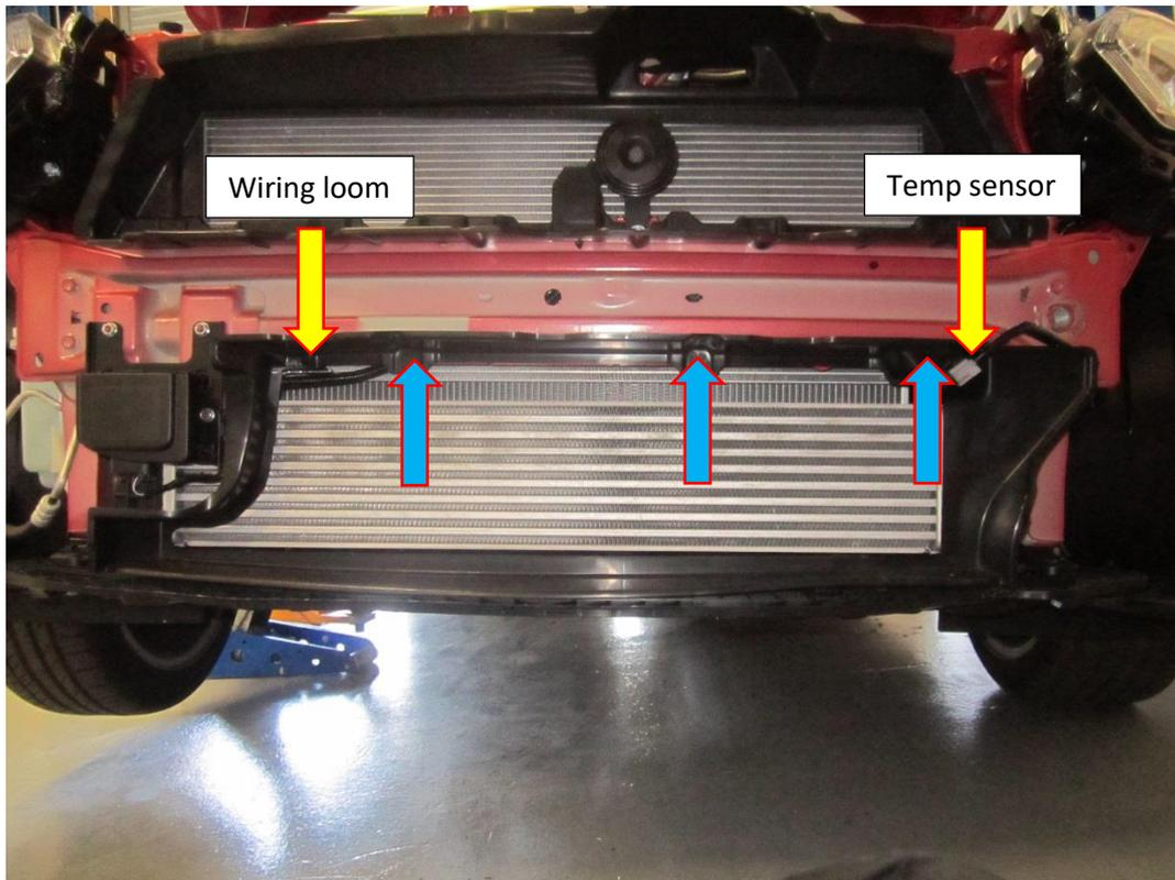
6. Accessing the car from underneath there are plastic covers that will need to be unfastened, to do this remove ten Philips fasteners Philips crew driver two 10mm fasteners with a 10mm socket and ratchet drive.
