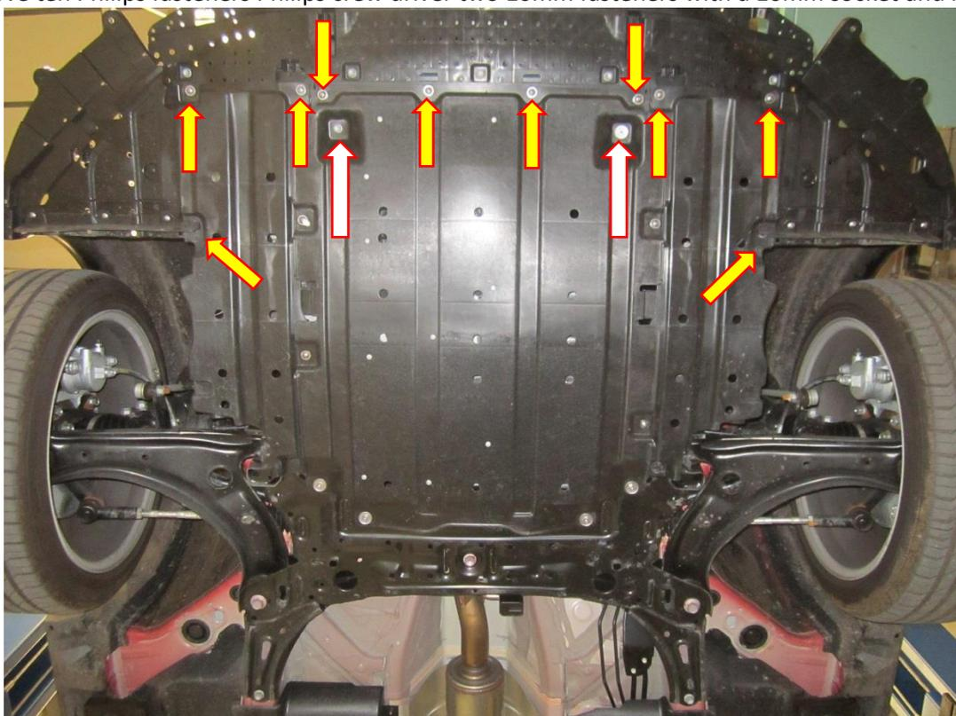
7. There are nine 10mm fasteners that now need to be removed from the front cover, use a 10mm socket and ratchet drive to undo them. Three of these fasteners which are shown in the picture by the four larger arrows are located underneath the side cover, there is enough slack to pull this side cover down and undo these 10mm fasteners. With this done pull the front cover forwards and push the two locating clips inwards and then you will be able to release the cover from the vehicle.
