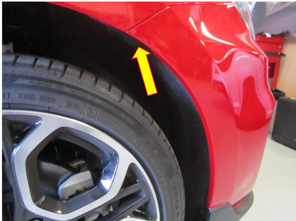
3. Raise the vehicle in the air via a ramp or with axel stands, so that you can access the eight Philips fasteners on the front valance of the bumper. Remove all eight fasteners with a screw driver, with done you will be left with two plastic fasters that also will need to be removed in the same way as step one.
