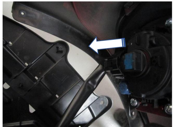
5. Now with the bumper removed you will see the OE intercooler, there is air ducting in front of the intercooler that needs to be removed. First remove the three plastic fasteners running along the top of the air ducting and unclip the air temperature sensor and the wiring loom with the use of a flat blade screw driver or trim tool. The ducting will not be able to be removed until steps six and seven are completed.
