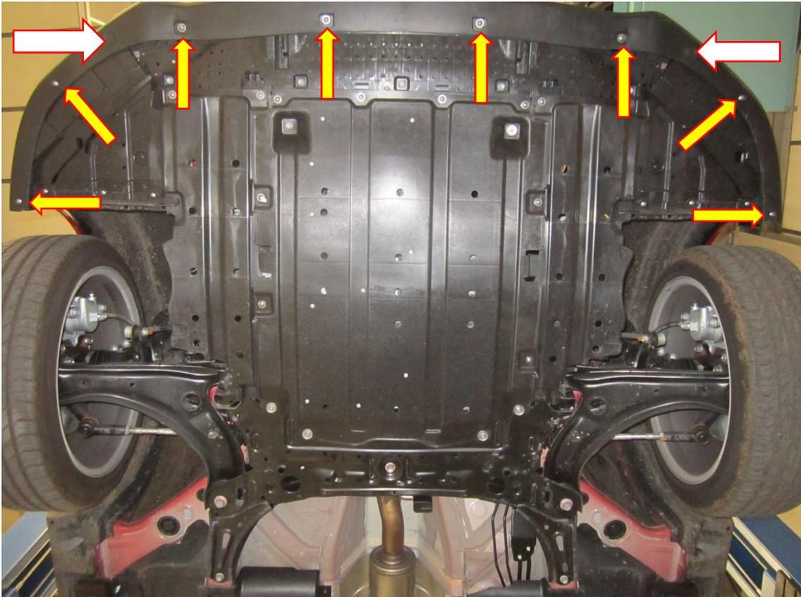
4. Pull each side of the bumper out wards starting from nearest to the wheel. The bumper will then pull away from the car, do not pull it completely off the car as the fog lights will need to be disconnected first. These simply un clip.
