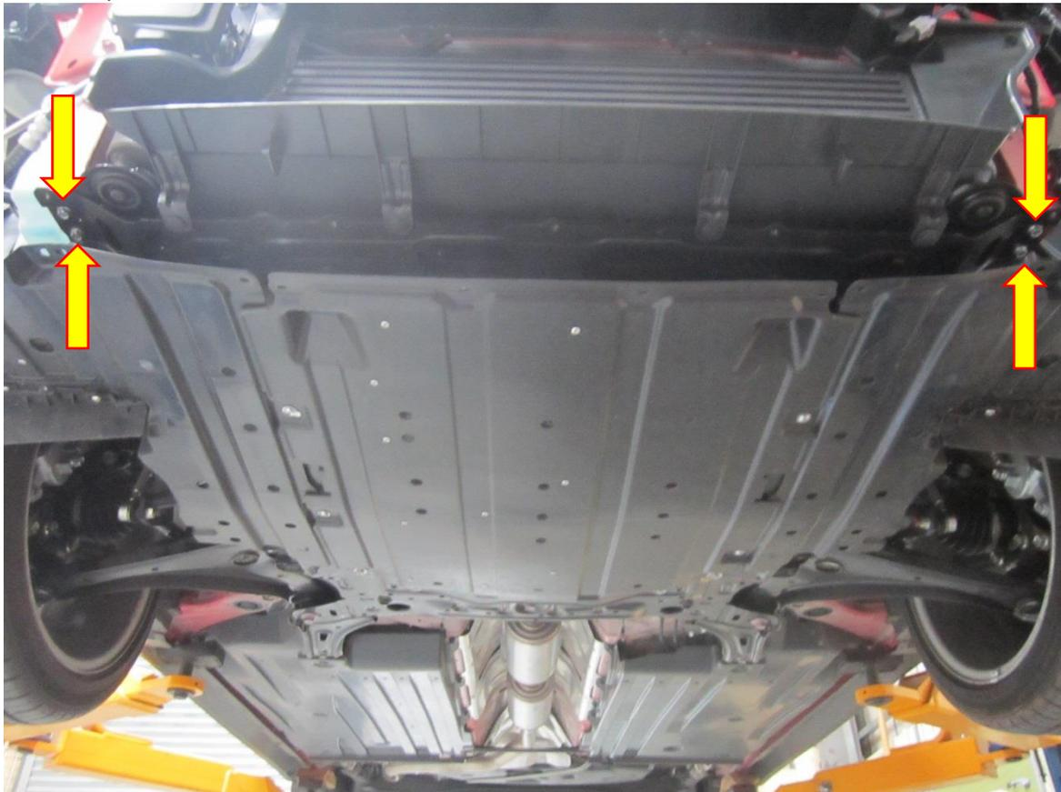
11. With the mounting bracket removed the next step is to undo the two hose clamps securing the rubber hoses to the inter cooler. They have 8mm fastenings which can be loosened off with an 8mm socket and ratchet drive or a flat blade screw driver.
