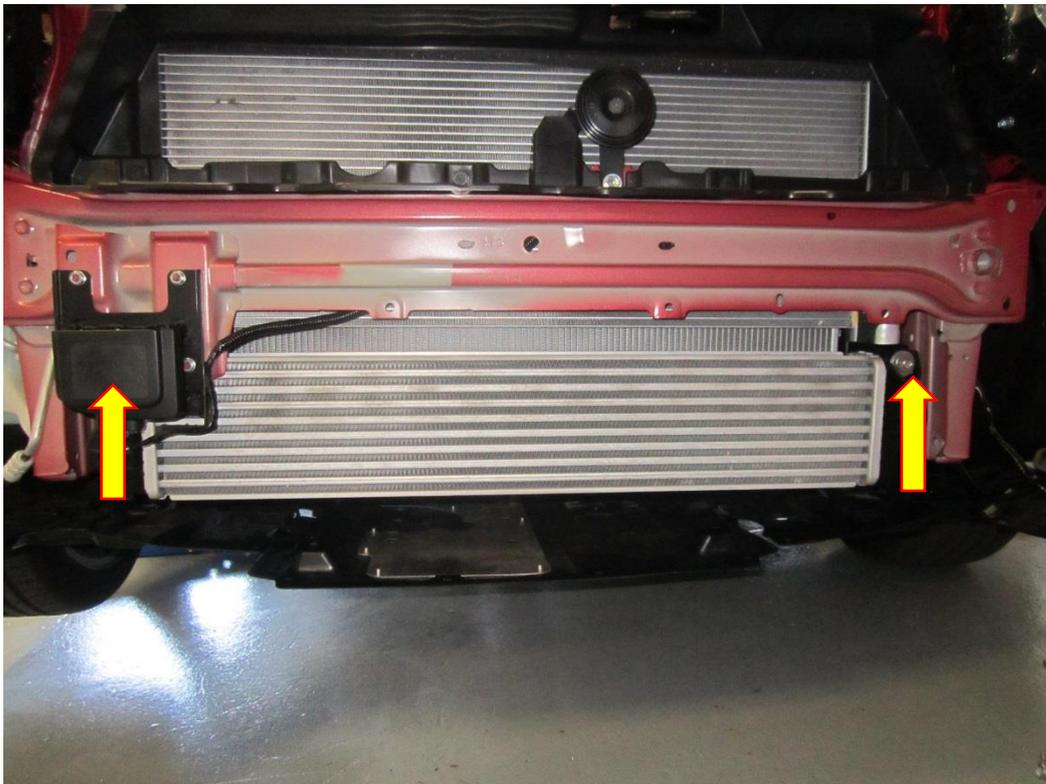
13. Now you will be able to install your new Forge Motorsport intercooler. Carefully angle the intercooler behind the ACC bracket and loosely re fit the two 10mm fasteners to hold the intercooler in place. You can then slide the hoses back on, locate the hoses as you can and then tighten the hose clamps up. Finally tighten the 10 mm fasteners.
