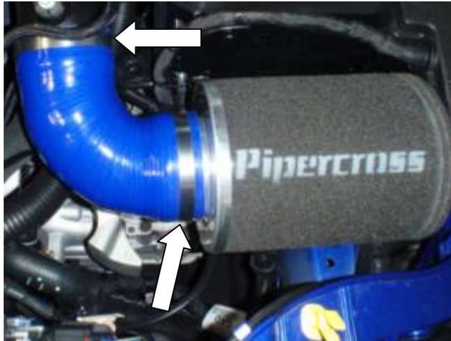
19. In the open end fit the Pipercross Filter and secure with the last jubilee clip.
