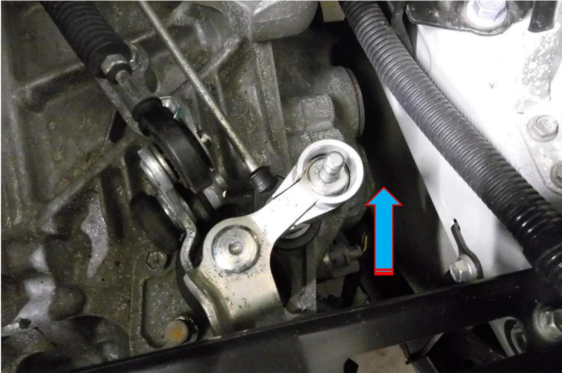
9. Place the machined locking nut from the FMSS5 kit through the gear box linkage pin and screw it to the FMSS5 body hand tight, then nip it up using a 16mm spanner or socket and ratchet.
