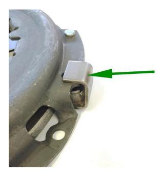
Remove 3off clips after bolting the Cover Assembly to the Flywheel
