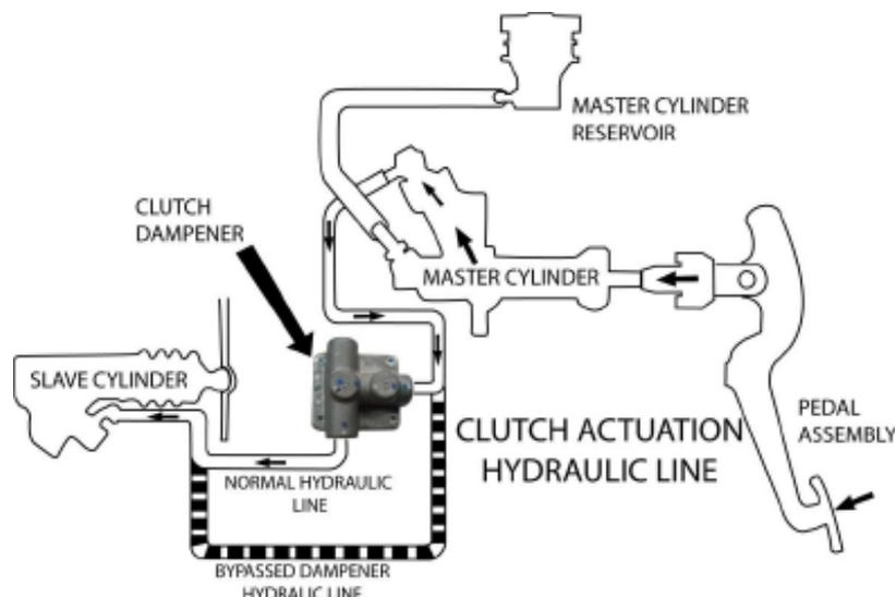
3. To confirm this is the case, bypass the clutch damper by using a suitable joiner tube from master cylinder directly to the slave cylinder. Then depress the clutch pedal to see if gear selection performance is sufficient.
