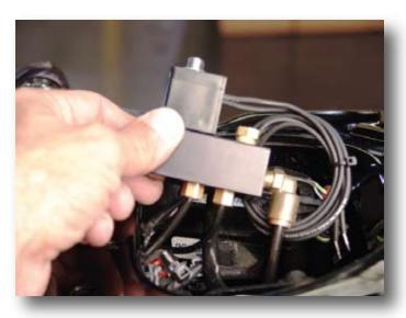
7. Install distribution manifold in the area under the seat and inboard of the battery and trim the ¼" line to appropriate length.. Connect the ¼" air line to the *push to connect* fitting. The manifold will distribute air to both shocks.
