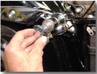
4. Install the bolt covers onto the shock absorber bolts. Lubricate the inside with a lube appropriate for o-rings. Gently press the cover on with a slight twisting motion until you feel it drawn solidly onto the bolt head and firmly seated.
