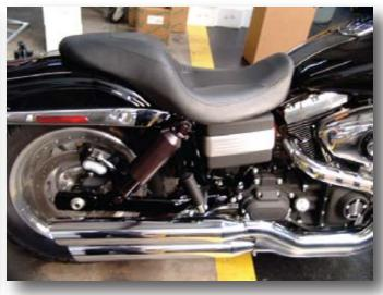
12. Reinstall the battery cover and seat, make sure the front tang is securely locked in the frame. With the system operational, check clearances around the tire and fender area and between the shock and belt guard, shim as needed.
