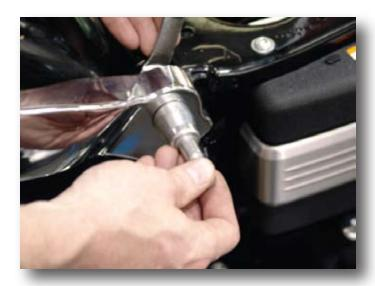
3. Loosen and remove the upper mounting studs.
