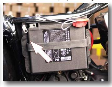
2. Use a 10mm wrench to disconnect the battery. ALWAYS DISCONNECT THE NEGATIVE (-) CABLE FIRST.
