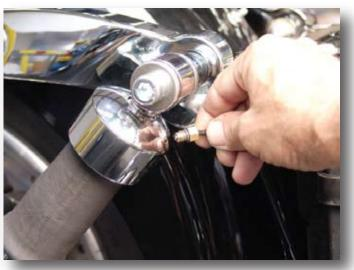
8. Use the smaller, 4mm air line and 4mm VOSS® fittings provided in the kit to connect the shock absorbers to the distribution manifold. Assembly instructions for the fittings are provided in the kit. VOSS® fittings use a o-ring to seal, use a 10mm wrench to snug the fittings, do not overtighten. NOTE: Fittings seal with an o-ring, DO NOT OVERTIGHTEN!
