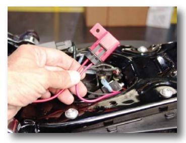
11. The preferred location for the fuse assembly is under the seat. Locate the universal fuse wiring assembly near the battery. Connect the red wire, (with the ring terminal), to 12 volt battery positive. Reconnect the battery cables, torque to 60-96 in-lbs. (6.8-10.9 Nm).
