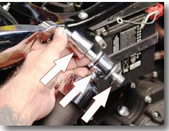
2. Locate and remove the two upper ½ X 4.5" socket head bolts from the kit. To install the upper shock bolt, install the washer on the bolt first, then slide the bolt through the top shock eyelet. Next, place the upper shock spacer bushing over the bolt. The larger diameter end of the bushing goes against the shock eyelet.
