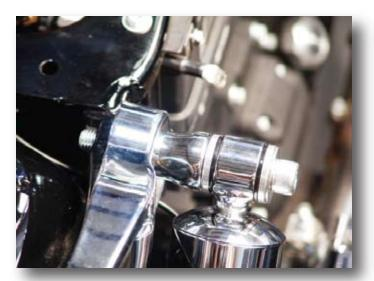
3. Install the upper shock bolt, it may be necessary to adjust the height of the bike to line up the upper shock bolt mounting hole. Apply two or three drops of blue (243) thread lock to the new shock bolts. Torque the upper shock bolts to 30-40 ft-lbs. (40.7-54.2 Nm)
