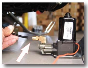
3. Preassemble the ¼" air line to the compressor by pushing one end of the tubing into the fitting leading from the air compressor. Route the air line along the lower right side of the frame to the rear of the transmission and up to the inboard side of the battery box.
