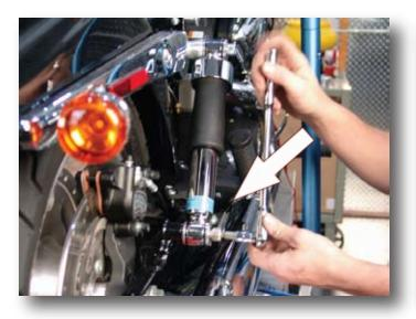
1. Locate and remove the two lower ½" X 2.5" socket head bolts from the bolt pack. Apply two or three drops of blue (243) thread lock to the new shock bolts. Tighten both lower shock bolts to 30-40 ft-lbs (40.7-54.2 Nm). NOTE: *Nuts will have to be reused on the bottom.*
