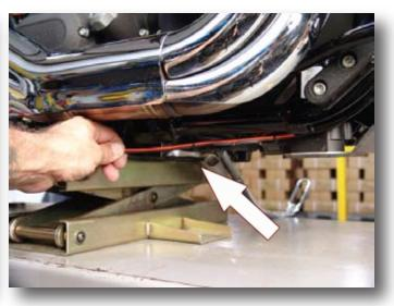
4. Route the orange power feed wire for the compressor along the same path that was used for the air line. Find a suitable ground for the black wire with the ring terminal.
