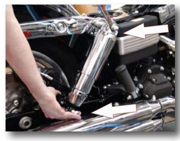
1. Loosen and remove the upper and lower shock hardware. Nuts are used on the lower mounting points. Keep these for installation.
