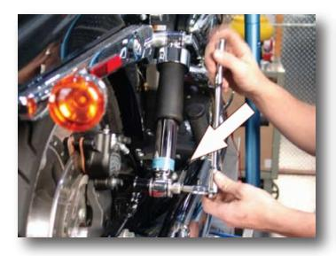
1. Locate and remove the two lower 1/2" X 2.5" socket head bolts from the bolt pack. Apply two or three drops of blue (243) thread lock to the new shock bolts. Tighten both lower shock bolts to 30-40 ft-lbs (40.7-54.2 Nm). NOTE: *Factory nuts will have to be reused.*
