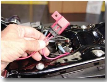
10. Refer to the included schematic for switch and relay wiring diagram. The preferred location for the fuse assembly is under the seat, near the battery. Connect the red wire with the ring terminal to 12V battery positive.
