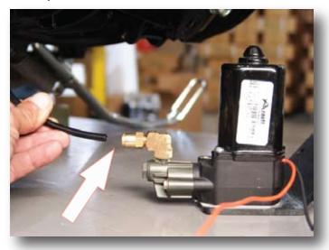
3. Preassemble the  $\frac{1}{4}$ " air line to the compressor by pushing one end of the tubing into the fitting leading from the air compressor. Route the air line along the lower right side of the frame to the rear of the transmission and up to the inboard side of the battery box.
