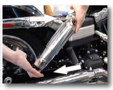
2. Carefully remove factory shock absorbers from the rear suspension.
