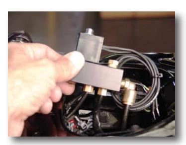
7. Once location of valve block has been determined, trim ¼" line to appropriate length. Install solenoid valve block in the area under the seat and inboard of the battery. Connect the ¼" air line to the *push to connect* fitting. The valve block will distribute air to both shocks.
