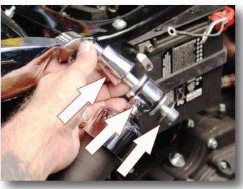
2. To install the upper 4.5" shock bolts, install the washer on the bolt first, then slide the bolt through the top shock eyelet. Next, place the upper shock spacer bushing over the bolt. The larger diameter end of the bushing goes against the shock eyelet.
