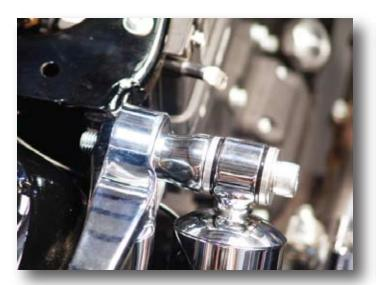
3. Install the upper shock bolt, it may be necessary to adjust the height of the bike to line up the upper shock bolt mounting hole. Re-using the factory nuts, torque the upper shock bolts to 30-40 ft-lbs. (40.7-54.2 Nm)
