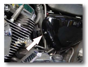
9. The location of the switch is the installers option, an example of a good location would be in the left side cover as shown.
