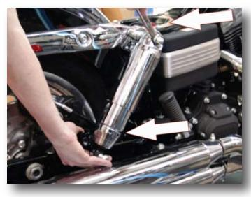
1. Loosen and remove the upper nut and lower shock bolt. Nut is used on the lower left side. Keep nut for installation.
