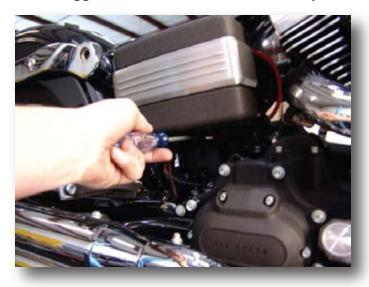
1. Remove the battery cover on the right side of the bike.
