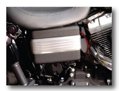
11. Once the system is operational, check all hose connections for leaks with a soap and water solution. Reinstall the battery cover.
