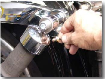
8. Use the smaller air line and 4mm VOSS® fittings provided in the kit to connect the shock absorbers to the solenoid valve block. Assembly instructions for the fittings are provided in the kit. VOSS® fittings use a o-ring to seal, use a 10mm wrench to snug the fittings, do not overtighten. NOTE: Fittings seal with an o-ring, DO NOT OVERTIGHTEN!
