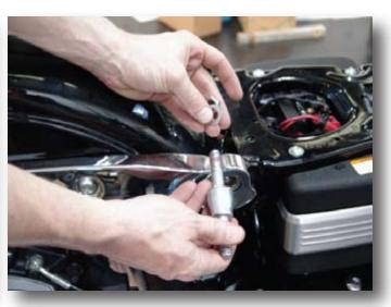
4. Remove nut, washer, and stud from the bike. Keep hardened washer and nut for installation of new shocks.
