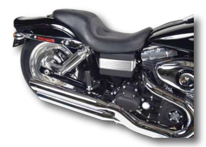
13. With the system deflated, roll the bike back and forth checking for any rubbing of the tire on the fender. Be sure to check the center and sides of the tire for contact. Also check the left side shock for interference with the belt guard, space as needed with washers.
