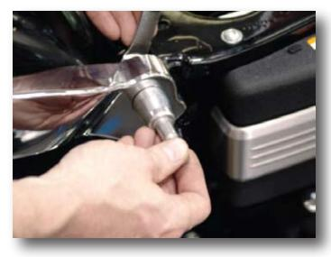
3. Loosen and remove the 1/2" nut located on the back side of the upper mounting stud.
