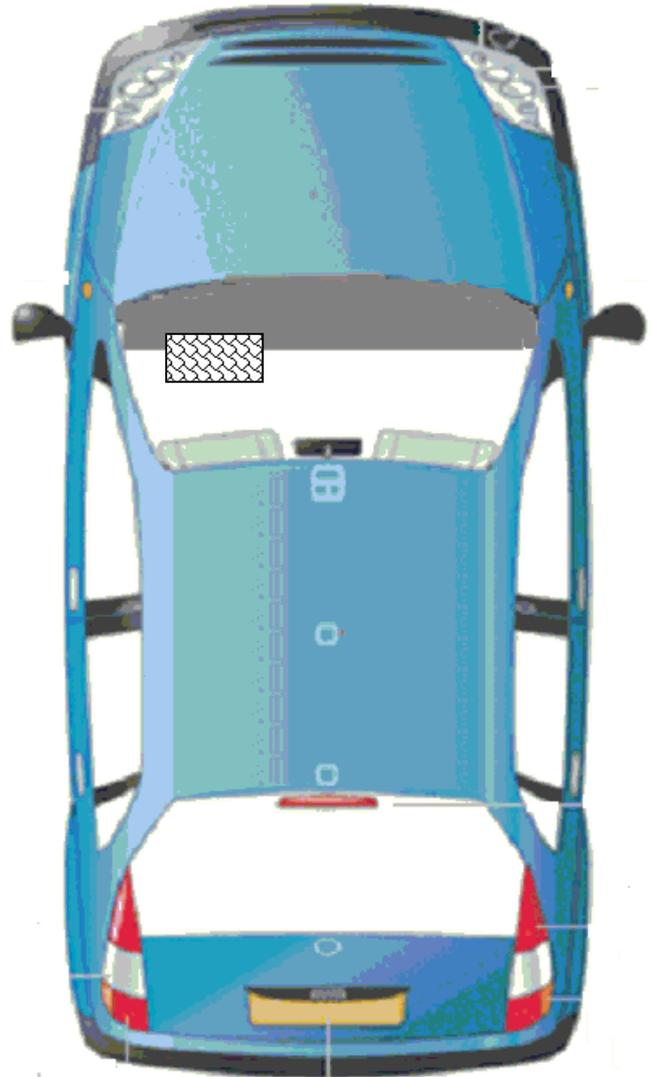
1. The Cabin Filter can be found under the glove compartment.
