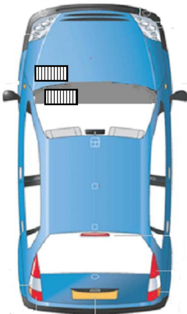
1. The first cabin filter is located between the glove box and passenger footwell. Remove trim to access the filter.
