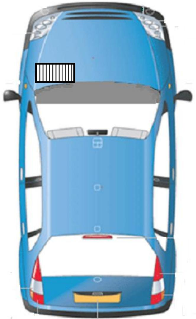
1. The cabin filter is located in the engine compartment in the nearside scuttle area.
