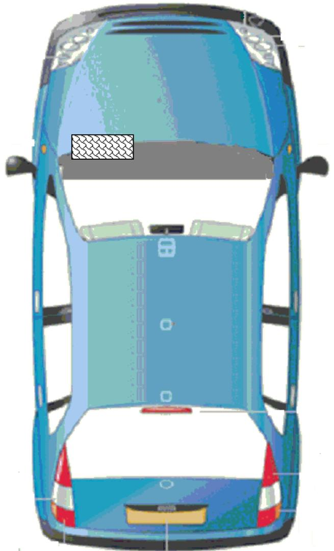
1. The Cabin Filter can be found in the engine compartment near the bottom of the windscreen.
