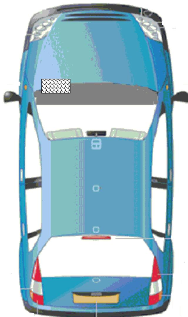
1. The Cabin Filter can be found on the passenger's side of the engine compartment just underneath the windscreen.
