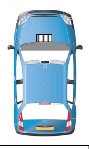
1. The cabin filter is located in the engine compartment in the scuttle area.
