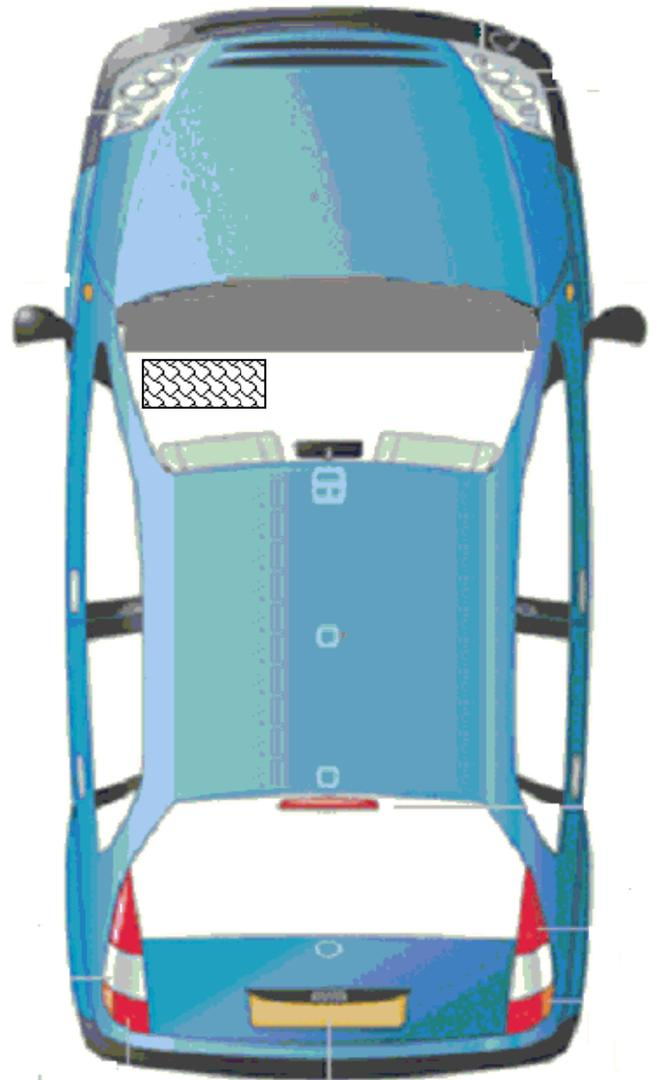
1. The cabin filter can be found on the passenger's side in the ceiling of the passenger's footwell
