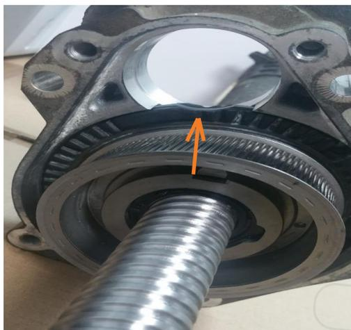
4. To start assembling the motor, carefully position the black plastic bearing. The position of the notch should be parallel with the housing as shown below. Please note this bearing will only move in an anti-clockwise rotation.
