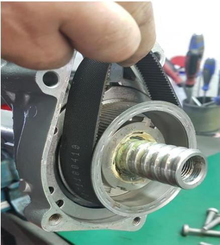
6. Carefully re install the drive belt, ensure the belt teeth are seated correctly.
