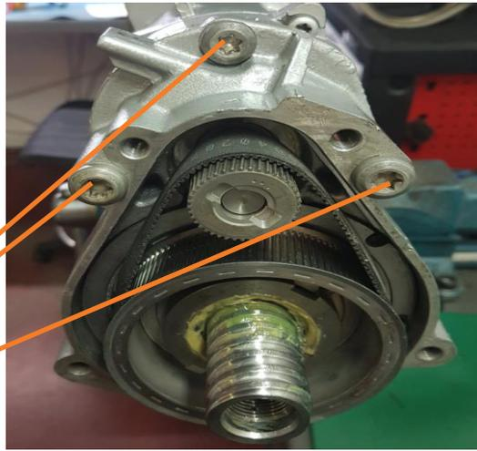
8. Screw the motor in position.
