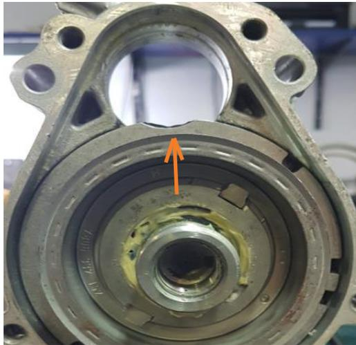
5. Re install the washer. The washer must be positioned to match the same notch as the black plastic bearing.
