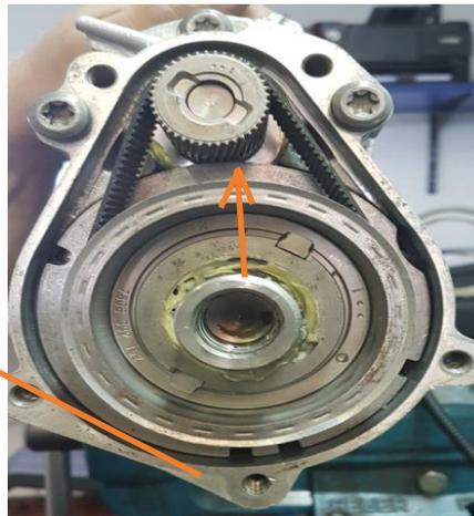
10. Place the locking pin in position and gently tap to lock the washer and black plastic bearing into position. NB: check there is sufficient clearance between the teeth of the motor and the washer
