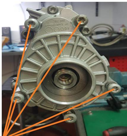
11. Re install the housing, and secure in place with 5 screws
