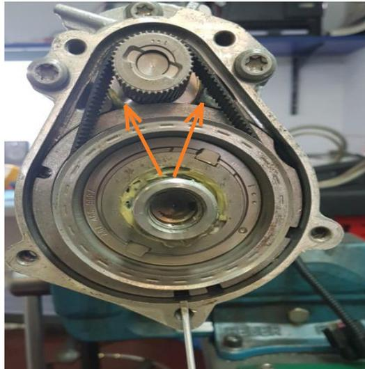
9. Using a screw driver turn the washer and black plastic bearing in a clockwise rotation until the belt is tight.
