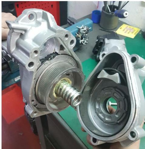
1. Remove part of the housing by removing 5 screws, keep the screws safe for later use
