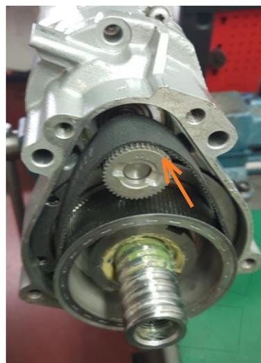
7. Hold the belt and insert the motor through the housing. Slide the belt over the teeth on the motor.
