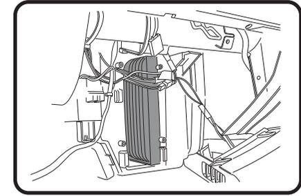
3: Hold wires away from front of housing, Pull used filter out from housing and replace with new Ryco RCA104P filter and re-assemble all previously removed components.
