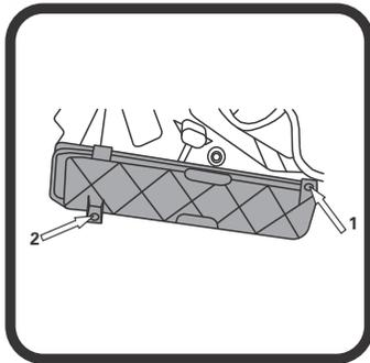
② Unlock in 2 places as shown, remove filter cover.
