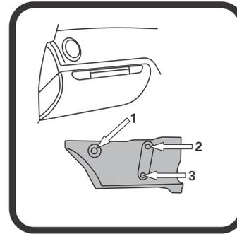
① Filter located under glovebox, remove panel by unlocking in 3 places as shown.
