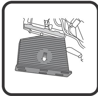
③ Pull dirty filter out to remove, push new Ryco filter into housing.
