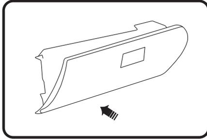
1. The cabin air filter is located behind the glove box compartment, it will have to be removed to gain access to the cabin air filter.
