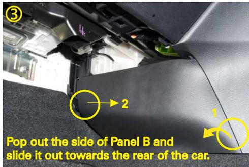
Pop out the side of Panel B and slide it out towards the rear of the car.
