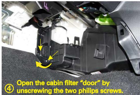
Open the cabin filter "door" by unscrewing the two philips screws.
