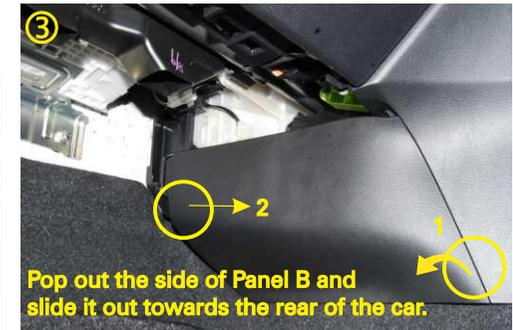
Pop out the side of Panel B and slide it out towards the rear of the car.
