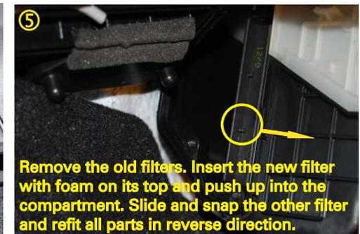
Remove the old filters. Insert the new filter with foam on its top and push up into the compartment. Slide and snap the other filter and refit all parts in reverse direction.
