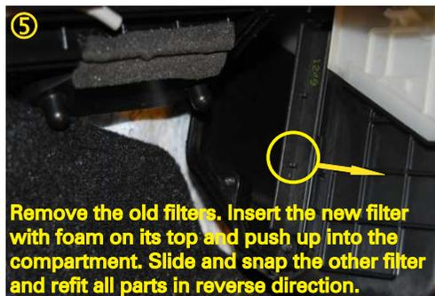
Remove the old filters. Insert the new filter with foam on its top and push up into the compartment. Slide and snap the other filter and refit all parts in reverse direction.
