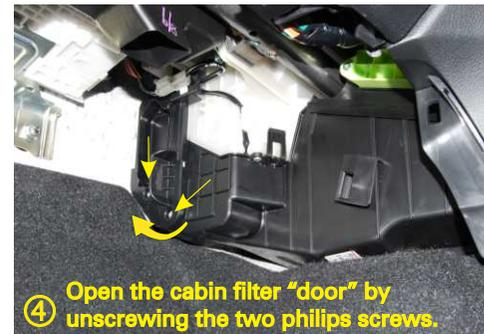
Open the cabin filter "door" by unscrewing the two philips screws.
