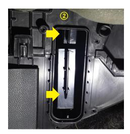
Once the cabin air filter housing lid is out of the way, the filter will be accesible. Pull the first filter out and then reach for the second one. Pay attention on how the filters sit in and replicate this with the new ones, making sure they are placed in the right air flow direction and lastly refit the housing lid.
