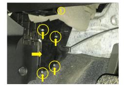
The cabin air filter location is on the drivers side footwell at the far end of the centre console. To access the filter undo the 4 screws shown in the picture with a Phillips screw driver and remove the housing lid.
