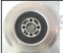
Picture of a new TVD. The dampening insert is in one piece with no cracks or imperfections.
