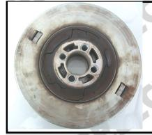
Picture of a WORN TVD (Torsional Vibration Damper or 'bottom pulley')
