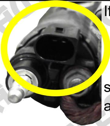
If the starter motor you are returning for surcharge credit shows signs of a broken plug/damaged plug this will **not** be accepted for full surcharge credit. Please check before supplying the new replacement alternator and accepting any old unit.
