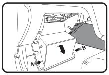
1: Open glove box, push each side of glove box (A & B) to release catches, glove box can then be rolled down to 180° position. Unclip trim panel (push / pull clips) (C) to reveal hidden screw.
