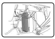
3: Hold wires away from front of housing, Pull used filter out from housing and replace with new Ryco RCA104P filter and re-assemble all previously removed components.
