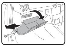
1: Open glovebox, remove screw and washer, then remove the glovebox.
