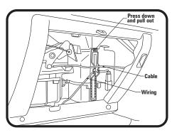
2: Remove cable and wiring from filter cover plate, push down and pull out to remove cover plate.
