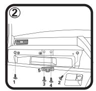
Open glove box, Undo 4 screws at top of glove box as shown, screws 3 & 4 retain staple (5) for glove box lock, lower glove box to access filter housing, Disconnect glove box light from back of glove box.
