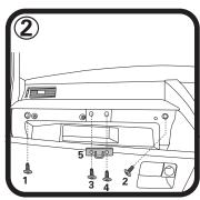
Open glove box, Undo 4 screws at top of glove box as shown, screws 3 & 4 retain staple (5) for glove box lock, lower glove box to access filter housing, Disconnect glove box light from back of glove box.
