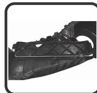
③ Place filter cover into the housing
