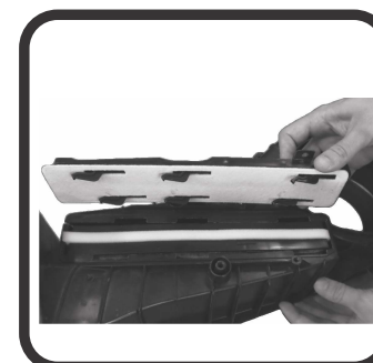
② Place the filter panel on the filter cover. Make sure the panel filter holes fit to the hooks.
