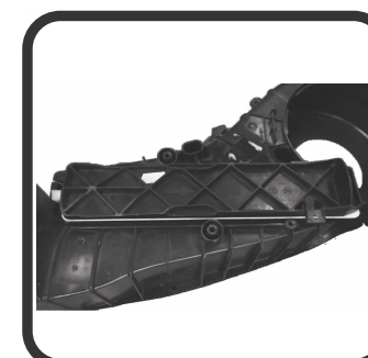
③ Place filter cover into the housing
