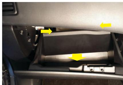
With the strut unclipped, proceed to release the glove box from its securing hinge. Simply apply some pressure to the far upper corners towards the inside of the compartment as indicated in the pic and slowly drop the unit.
