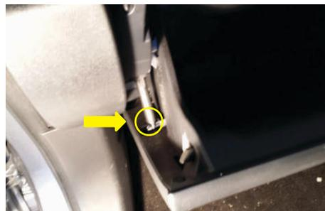
The cabin air filter housing is located behind the glovebox. To gain access, the glovebox has to first be removed. Remove objects from compartment and unclip the strut shown in pic above.
