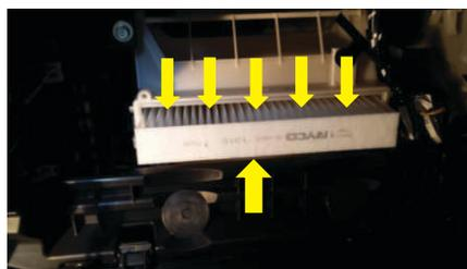
Insert the new filter in the right air flow direction. Look for arrow on one of the sides of the filter to identify air flow direction. Re-fit all components in reverse order.
