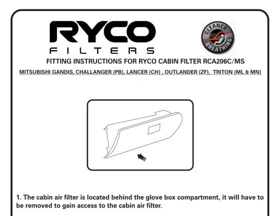
2. Open the glove box and press inwards on both top corners so that the retaining lugs can be bypassed then let the compartment completely drop.
