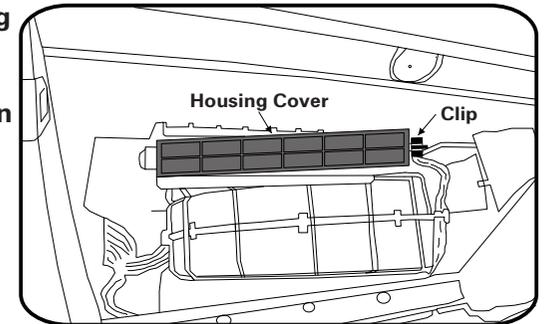
3. Remove old filter and push new filter into the housing. Refit housing cover and glove box. Dispose of used filter correctly.
