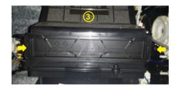
With the glove box unit out of the way the cabin filter housing is easily recognisable facing right at you. Proceed to unclip both sides as shown and slide it out.
