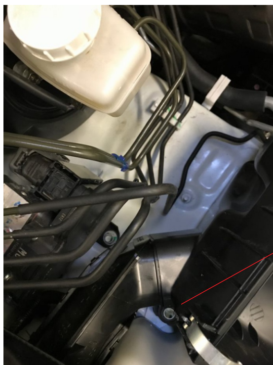
FIG. 8b AIRBOX MOUNTING OEM BOLT/WASHER REMOVAL
