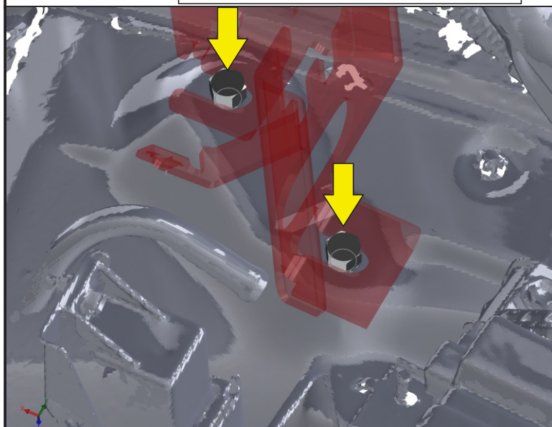
FIG. 4c FB9810FC BRACKET INSTALLATION
