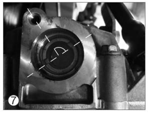
Using a suitable counter hold (such as HAZET 2540-2 Camshaft Holding Tool) rotate the camshaft to the position shown in picture 7.
