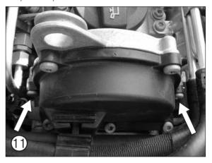
Screw HAZET 2588–22 timing cover guide pins into two of the threaded holes on the cylinder head, (see picture 11).
