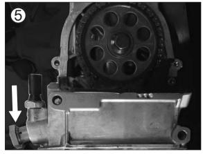
Remove the timing chain cover. Remove the timing chain tensioner.
