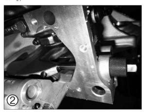
Carefully rotate the crankshaft pulley in the direction of engine rotation until the web of the crankshaft contacts HAZET 2588-21 crankshaft locking pin.
