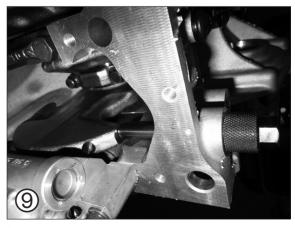
Carefully rotate the crankshaft pulley in the direction of engine rotation until HAZET 2588-21 crankshaft locking pin contacts the web of the crankshaft
