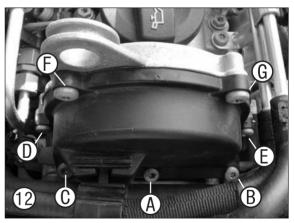
Remove HAZET 2588-22 timing cover guide pins.
