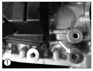
The threaded hole for the crankshaft locking pin is located at the rear of the engine block, and towards the timing chain cover.
