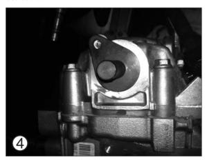
If it is not possible to correctly install HAZET 2588-20 camshaft locking tool then the engine timing requires adjustment.
