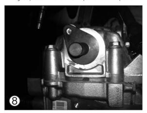
Install HAZET 2588-20 camshaft locking tool and secure in place with a suitable bolt.
