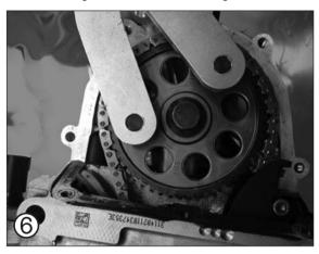
Using a suitable counter hold (such as HAZET 2540-2 Camshaft Holding Tool) remove the camshaft central bolt.
