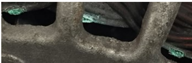
Close up of damaged stator wires due to ingress.
