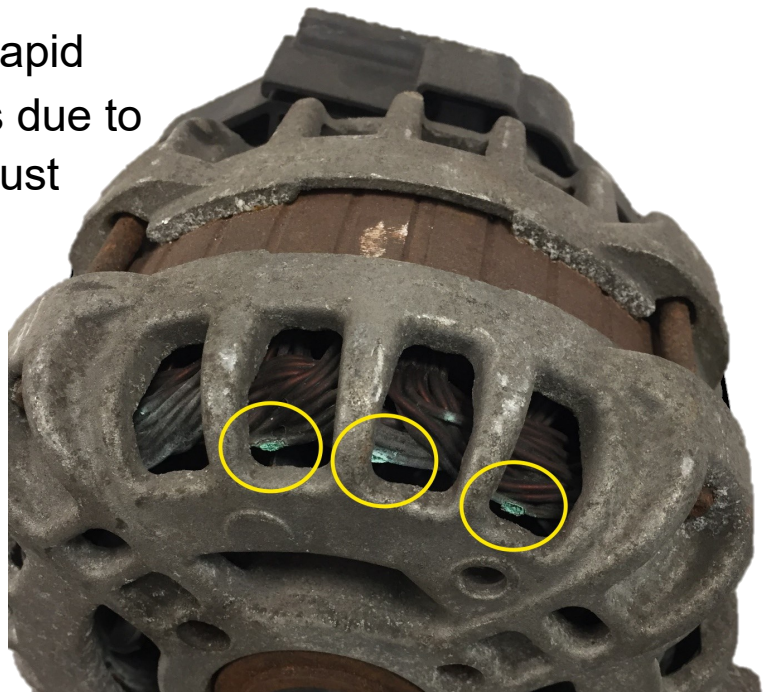
Close up of damaged stator wires due to ingress.
