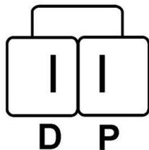
AEB1409 – This alternator is externally regulated through the vehicle ECU and the voltage is controlled by the ECU. This part cannot be interchanged with an AEA2238 alternator.
