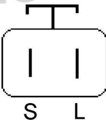
AEA2238/AEK2314 – This alternator is internally regulated. The charging process is controlled by the alternator. This alternator can be identified by testing the wires on the wiring harness to the alternator. The 'S' terminal should show a permanent battery voltage and the 'L' terminal should show voltage with the ignition switched on. This part is also commonly affected by burnt/rusty pulleys or belt slip. Please inspect your old unit for signs of this failure and ensure the belt is replaced.
