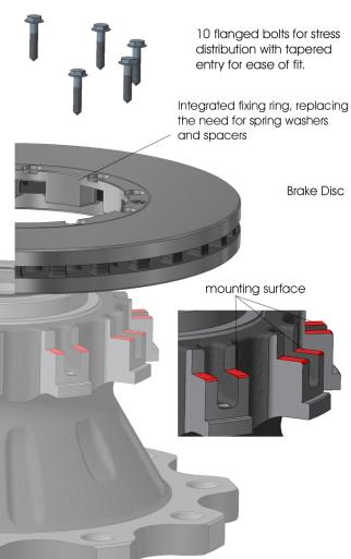
The original design is mounted on a small surface area and is prone to excessive wear. Excessive wear to this area can cause the disc to become loose.
