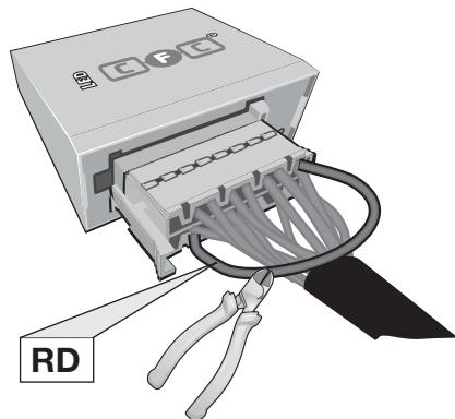
**Pin 11 and Pin 2 disconnected**
