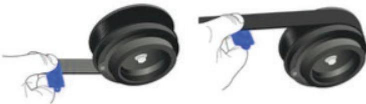
With the engine off, press the gauge ribs into the belt grooves using gentle pressure to hold the gauge against the belt and seat the ribs.
