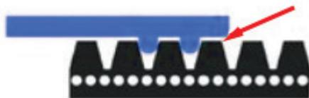
The gauge ribs will contact the sides of the belt material and the body may rest slightly above the belt surface.
