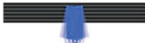
If the gauge can be moved within the ribs, the belt requires replacement.
