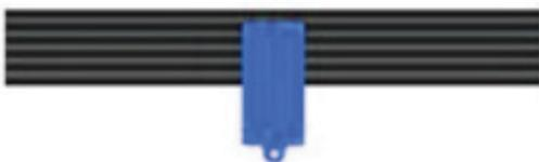
When the gauge remains tightly seated and resists movement, the belt has sufficient life left.
