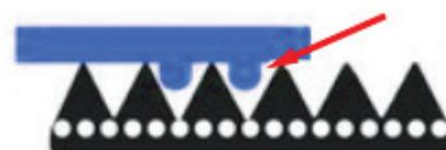
The gauge ribs will not contact the belt material and the gauge body will rest flat on the belt, allowing movement in the tool.
