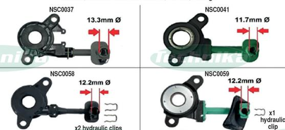
When replacing cylinders, please ensure the diameters of the hydraulic connections on the old and new parts match. If the wrong hydraulic connection is installed, it will cause leaks and system failure.
