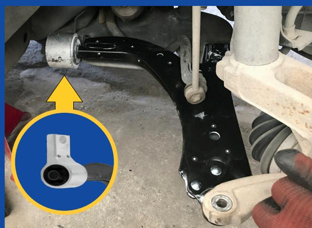
Apply sufficient force to push the wishbone bush into the location hole. This will align the bushes and the ball joint for fitment.
