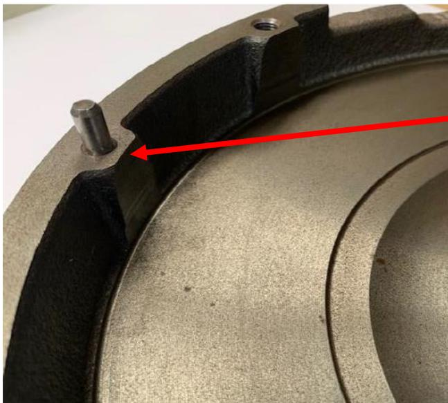
Pressure needs to be applied to the disc to clear this section of the flywheel.
