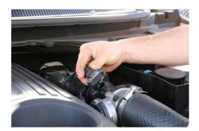
• Gently pull out the factory fitted MAP sensor and place in a safe location.
