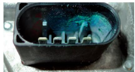
Built-in plug with traces of corrosion
