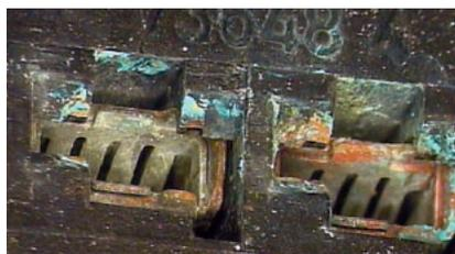
Coupling with traces of moisture and corrosion
