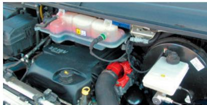
Regulating throttle (highlighted in red) in the engine compartment of an Iveco Daily 3.0 l
