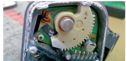
View of the interior of a damaged regulating throttle
